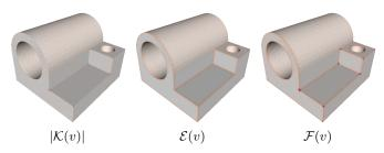
Fig. 8. From left to right Gaussian curvature  $|\mathcal{K}|$ , feature edge intensity  $\mathcal{E}$  and combined feature intensity  $\mathcal{F}$ , with higher intensities in red.
