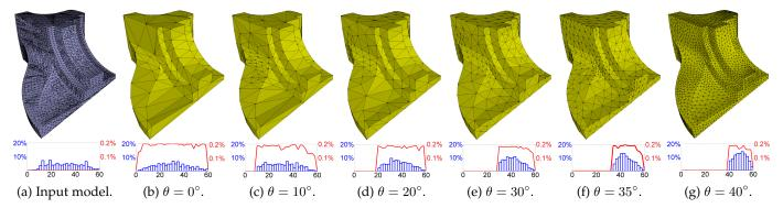
Fig. 1. Examples of surface meshes generated with our approach. The input model (a) has 7.2k vertices. From (b) to (g) are the results with different minimal angle threshold  $\theta$ . The angle distributions and their corresponding approximation error are shown below each result, in blue bars and red curves respectively. The error-bound threshold  $\delta$  is set to 0.2% of the diagonal length of the input's bounding box (%bb).
