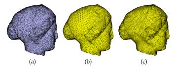
Fig. 16. Egea models with/without executing Alg. 2. we set  $\theta=40^\circ$  and  $\delta=0.20(\%bb)$ . The input (a) has 8.3k vertices. The result with Alg. 2 enabled has 4.2k vertices (b), and spends 330 seconds; the result with Alg. 2 disabled has 7.6k vertices (c), and spends 133 seconds.
