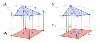
(a) Stratified samples on  $M_R$  (b) Stratified samples on  $M_I$  and their shortest links to  $M_I$ . and their shortest links to  $M_R$ .
