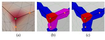
Fig. 9. Visualization of  $\mathcal{F}(v)$  in (a). The color of v's Voronoi cell represents the number of important neighbors, with red=0, blue=2, purple=3 and gray=degree(v) is shown in (b) and (c). A wrong classification based on solely feature intensity in (b) is corrected by additionally checking importance of edges in (c).
