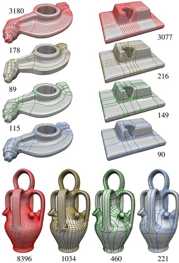
Figure 20: Comparison of automatic connectivity optimization approaches: The non-optimized separatrixes are shown in red, while those resulting from [BLK11], [TPP\*11] and [CBK12] are shown in gold, green, and blue, respectively. For a quantitative comparison, the number of resulting quadrilateral patches is indicated.
