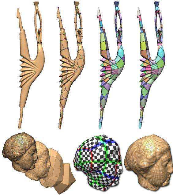
Figure 5: Top: different phases composing [DBG\*06]; given a triangle mesh, an initial Morse-Smale complex is extracted, then boundaries are improved through a sequence of relaxation steps, this finally allows to gather a high quality quadrangulated model. Bottom: The step composing [DSC09]; a base domain is obtained through a sequence of simplification operations, original vertices were mapped to the base domain, then sampling the base domain is possible to gather a semiregular quad mesh.
