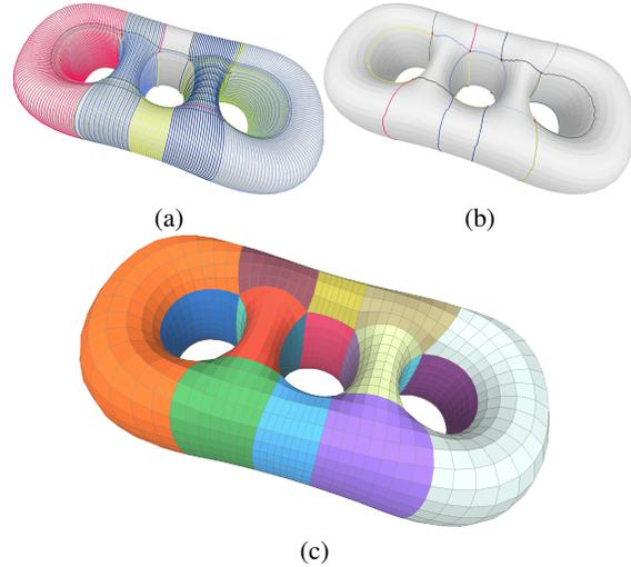
Figure 19: (a) A valence semi-regular quad mesh with just sixteen irregular vertices and an entangled graph of *separatrices* defining almost eight thousand domains in the base mesh; (b) by using [TPP\*11] the graph is disentangled to twenty-eight domains; (c) a semi-regular remeshing obtained by resampling the base mesh.
