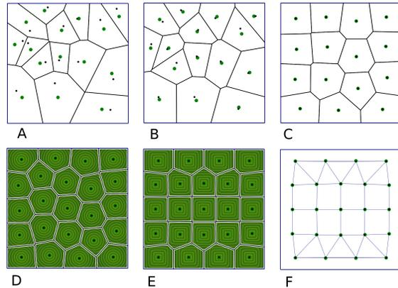
Figure 10: A: random sampling. The samples are shown in black and the centroids in green. B: result after one iteration of Lloyd relaxation. C: convergence of Lloyd relaxation. D: standard CVT (with  $L_2$  norm). E:  $L_p$ -CVT. F: quad-dominant mesh obtained from (E) by triangle merging.
