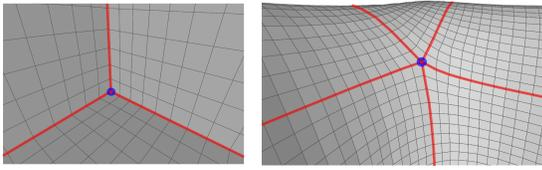
Figure 18: Left: three *separatrices* stemming from a valency 3 irregular vertex. Right: five *separatrices* stemming from a valency 5 irregular vertex. In a closed mesh, each separatrix is bound to end in another (or the same) irregular vertex.
